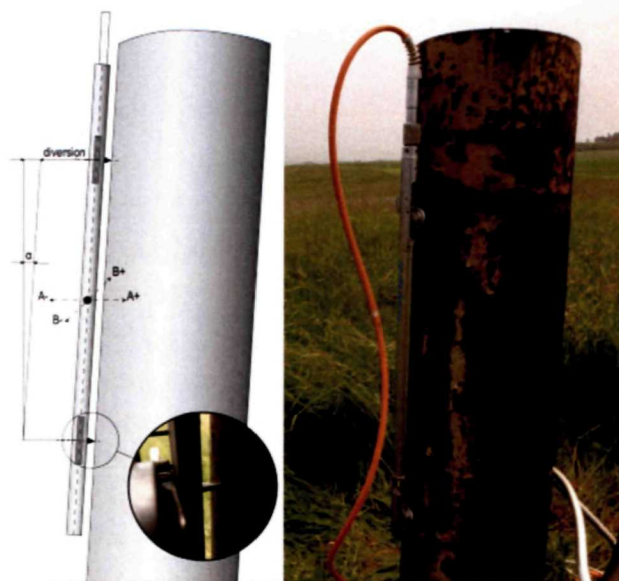
Fig. 7.8 Principle of measurements of change in angle of geodetic pillars by inclinometric probe
