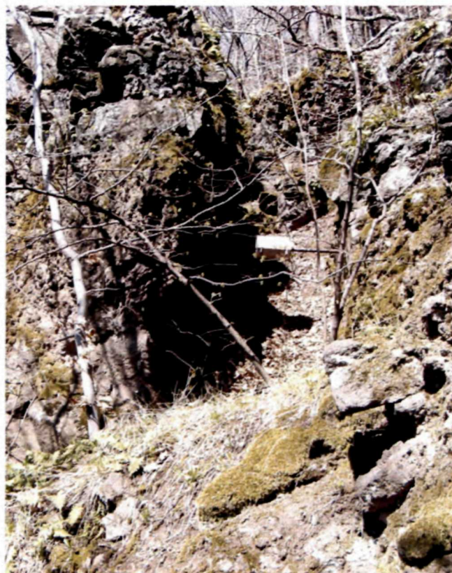
Fig. 7.24 Dilatometer TM-71 (KK-1) installed in the open crack between two (bottom and top) blocks at the western margin of the lava flow of the stratovolcano Střechový vrch
